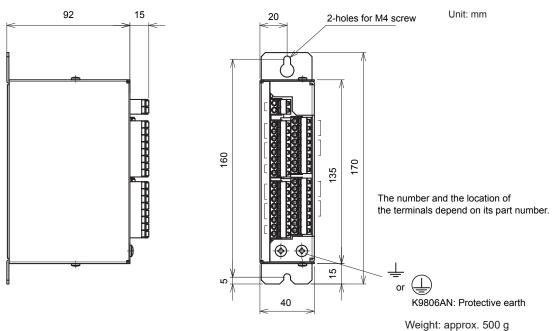
Note: Rack-mounted type should be installed vertically. The space between the converters/the signal interrupters with mark (\*) should be kept more than 10 mm.
