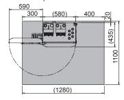
\*4: Required clearance needed for wiring.
