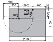
\*5: Required clearance needed for wiring.
