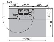
\*5: Required clearance needed for wiring.
