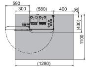
\*5: Required clearance needed for wiring.
