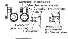
For FM-X, CSA-X (wiring connection: 3/4NPT)
